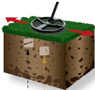
E.g. Passing the coil over an iron object close to the surface then over a good metal target (ring).
